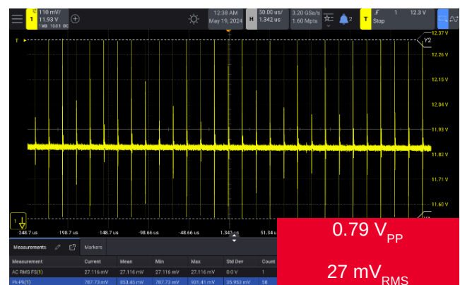
Figure 1. When comparing measurements taken on the Keysight InfiniiVision 3000G X-Series oscilloscope and the HD3 Series using the same probing setup, we find that the HD3 Series provides more accurate measurements. The HD3 features significantly higher vertical resolution with a 14-bit ADC and a low noise floor of 50 \mu V RMS . In contrast, the 3000G has 8 bits and a 250 \mu V RMS of noise. The difference significantly affects measurement accuracy.
