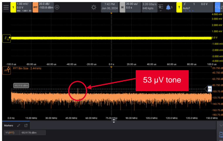
Figures 2a and 2b. Figure 2a (left) shows an extremely low-voltage tone on our fast Fourier transform (53 \mu V) thanks to the low-noise front end of the Keysight InfiniiVision HD3 Series oscilloscope. It is not even possible to see this tone on other oscilloscopes in this class because their noise floor is too high. If you cannot detect small tones that might interfere with the functionality of your supply, you cannot eliminate them. Figure 2b (right) shows the HD3 Series, engineered to have an extremely low noise front end.
