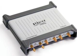
PicoSource PG900 Series Differential picosecond pulse generators
