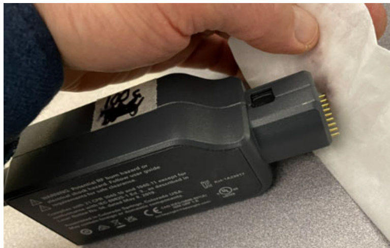
Figure 32 Cleaning probe pogo pins with IPA-saturated wipe
