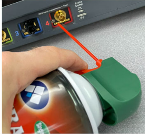
Figure 31 Spraying with duster
