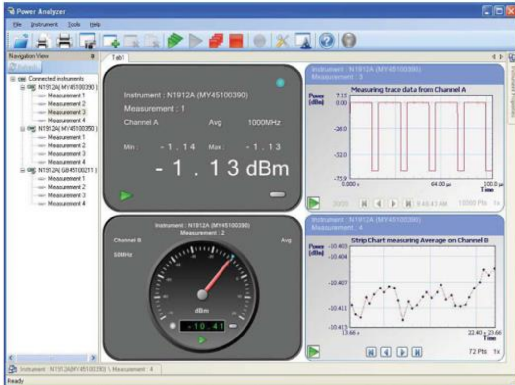
Figure 19. N1918A Power Analyzer
