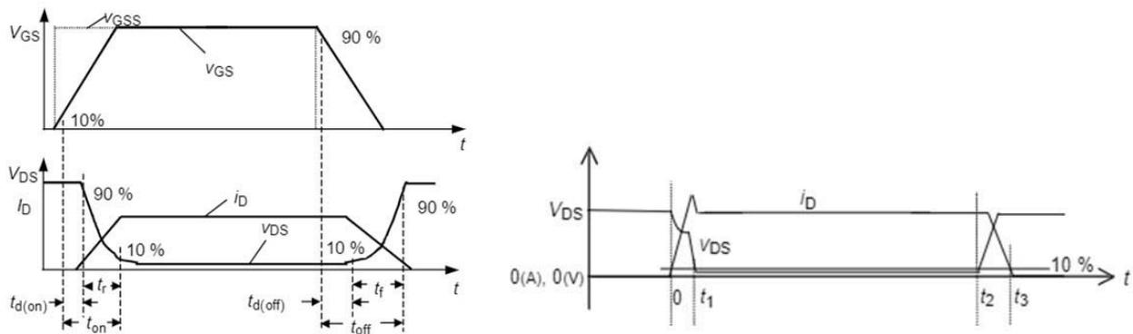
Figure 9. Waveforms and positions of switching times extractions according to IEC 60747-8
