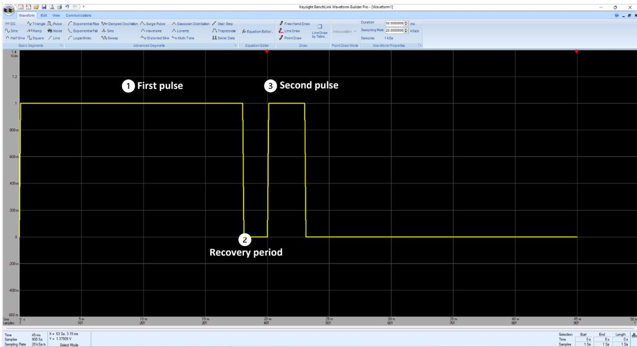
Figure 4. Double pulse signal display in the Keysight BenchLink Waveform Builder Pro application
