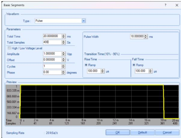
Figure 2. First pulse configuration and off-time setting
