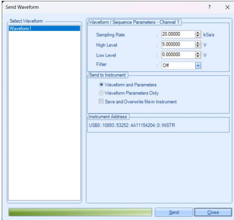
Figure 6. Send the waveform data to FG33532A
