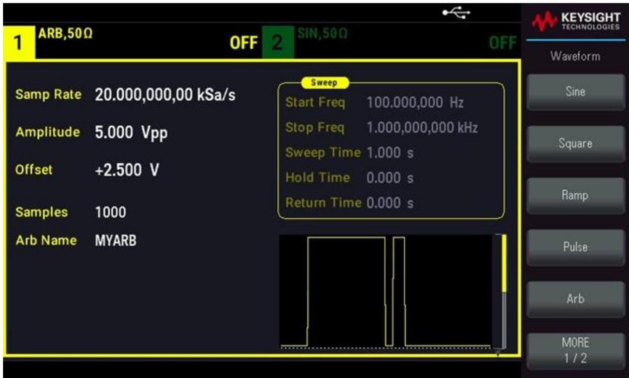
Figure 7. Waveform preview and parameters display on FG33532A
