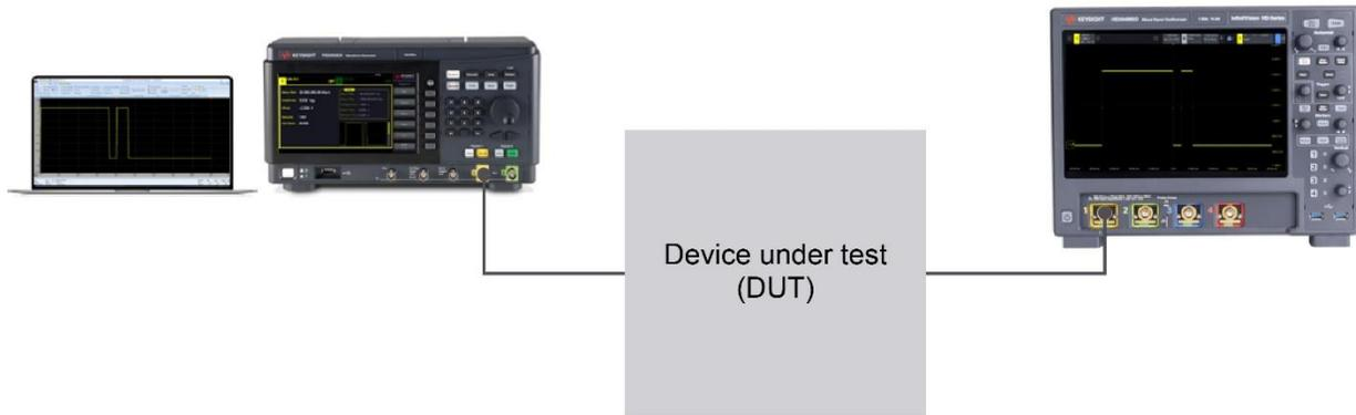
**Figure 1.** Instrument setup for double pulse testing
