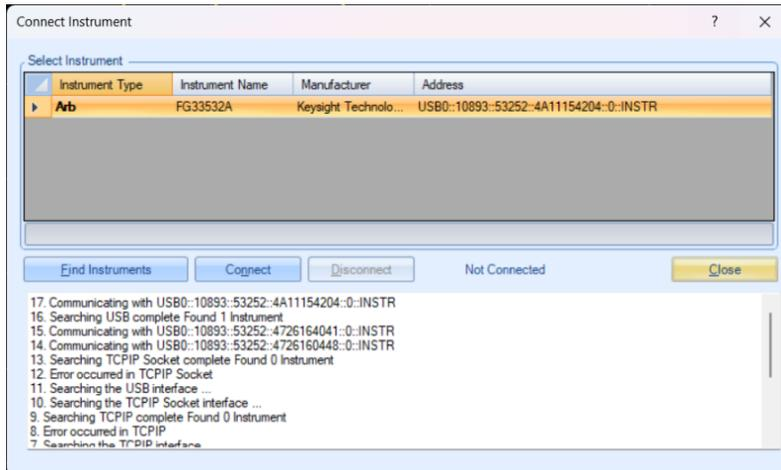
Figure 5. Connect the Keysight FG33532A function / arbitrary waveform generator before importing the waveform data
