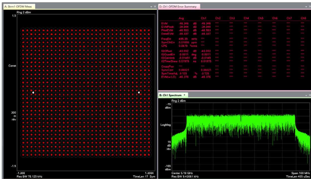
Figure 5.6. 802.11ax constellation diagram and error summary
