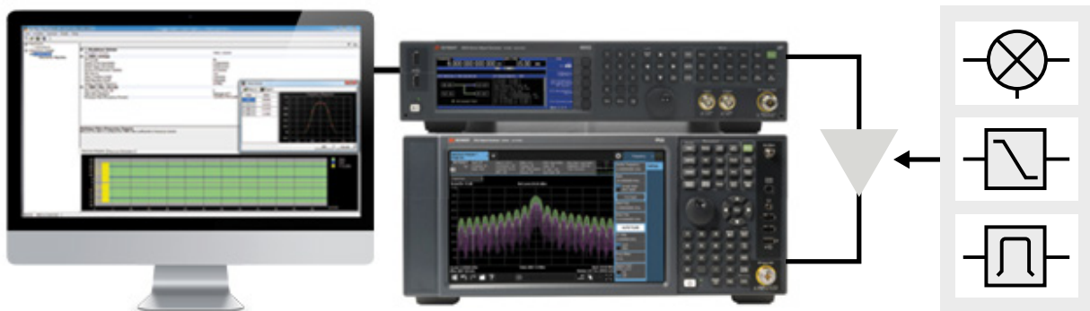
Figure 8.2. Typical component test configuration using Signal Studio with a Keysight X-Series signal generator and analyzer
