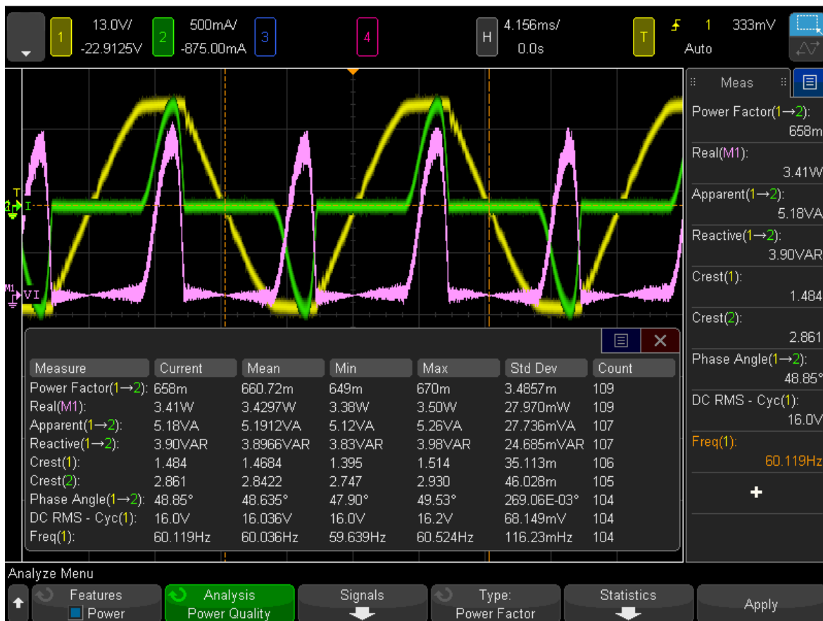
Figure 2. Automatic input power quality measurements performed by a Keysight oscilloscope
