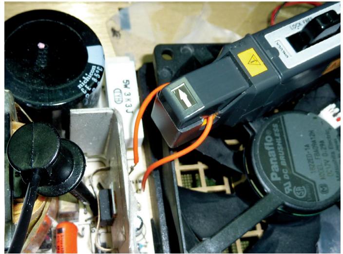
Figure 4. Creating a special current loop in your power supply to measure current.
