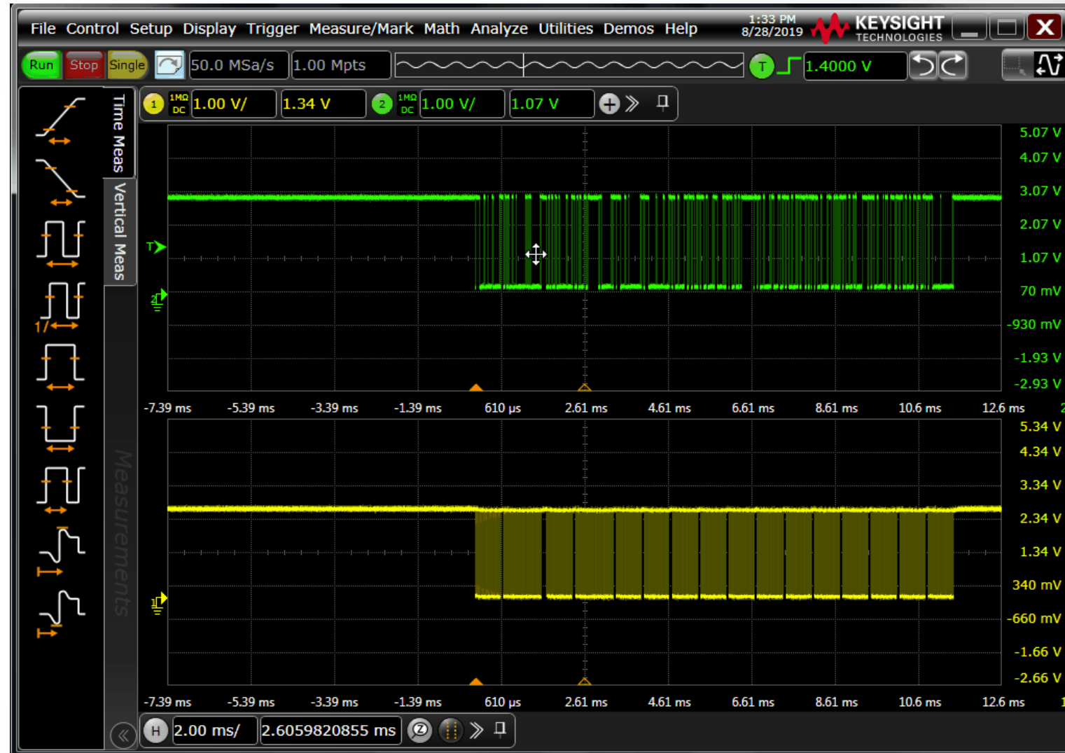
Example: Triggering on an I 2 C serial bus
