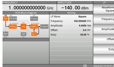
2. Press the F1 key to change the waveform when the LF output is activated.
