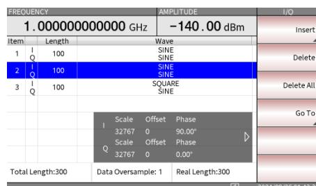
4. Use the scroll knob and arrow keys to select the waveforms for both channels I and channel Q and edit their corresponding parameter (including Scale, Offset, Phase, Duty, Symmetry), and edit Length for waveforms. Press the F6 key to apply it.
