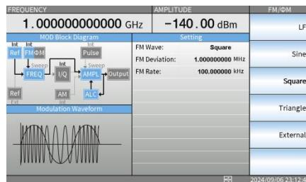
2. Press the F1 soft key to set the FM Deviation and press the F2 soft key to set the FM Rate.
