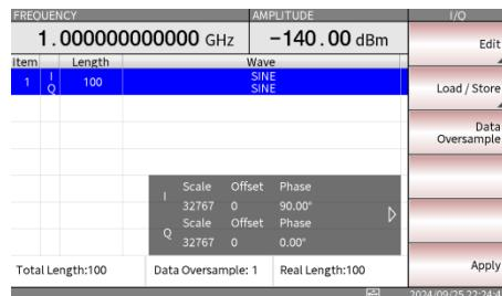
Insert Waveform 3. Press the F1 key to insert a ARB waveform.
