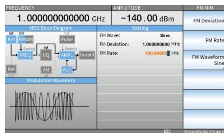
4. Use the left and right arrow keys to select the digit to be changed and then use the up and down arrow keys to increase or decrease the value of the digit to be edited.
