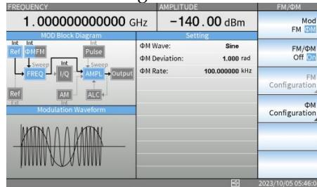
8. To change the ΦM modulation waveform, press the F3 key and select a wave you need. The following steps for changing waveform is similar to those indicated above in step 2 through step 6.
