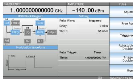
2. Press the F1 soft key and the F2 soft key to set the triggered waveform's Delay and Width, respectively.
