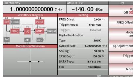
When a modulation mode is selected, the current modulation mode will be indicated in bold font. For example, if Digital Modulation is selected, option **Digital Modulation** will become bold.
