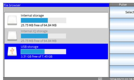
3. Turn the scroll knob to select the .pust file and press the Select key to open it.
