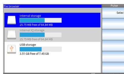
2. Turn the scroll knob to USB storage and then press the enter key.
