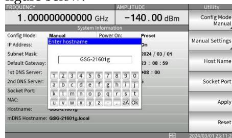
2. Use the arrow keys and the keys on the keypad to edit the host name and finally press the OK key on the left lower corner to apply the setting.
