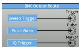
2. Press the F1 key to select the polarity of the trigger output and toggle between Pos and Neg polarity. If Neg is selected, you will see a small icon that looks like a small circle at the end of the route to indicate that the present output polarity is Negative.
