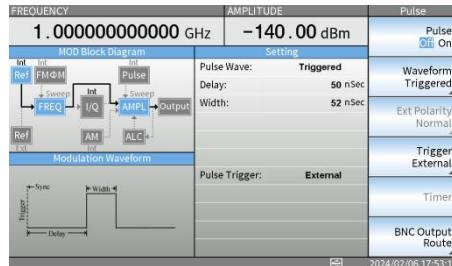
6. Press the F1 key to activate Pulse modulation. Press the F1 key again to disable Pulse modulation. When Pulse modulation is activated, the Pulse key will light on, and you will see the Pulse icon in the MOD Block Diagram turning blue, as shown in the figure below.
