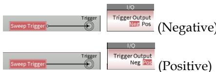
3. Press the F2 key to select which kind of BNC output route to trigger output. There are five types of BNC output routes available including Pulse Video, Pulse Trigger, Sweep Trigger, Sweep Run, and IQ Generator Trigger.
