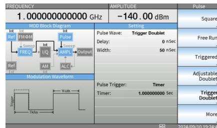
2. Press the F1 soft key and the F2 soft key to set the triggered doublet's Delay and Width, respectively.
