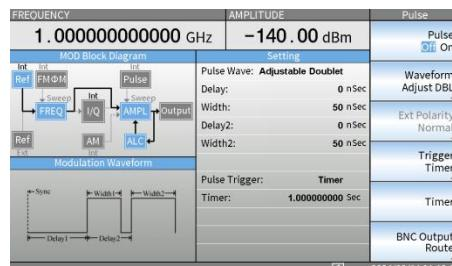
2. To set the pulse trigger to a Timer, Press the F1 key.
