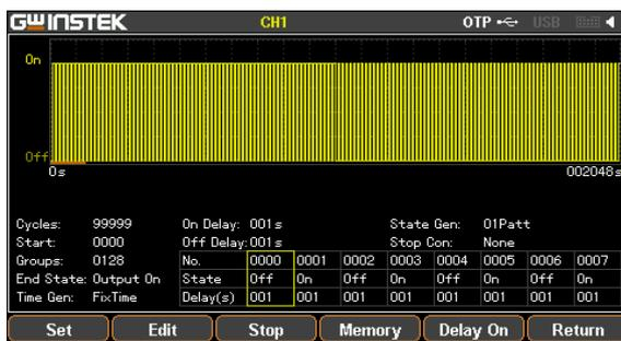
GPP series delayed waveform
