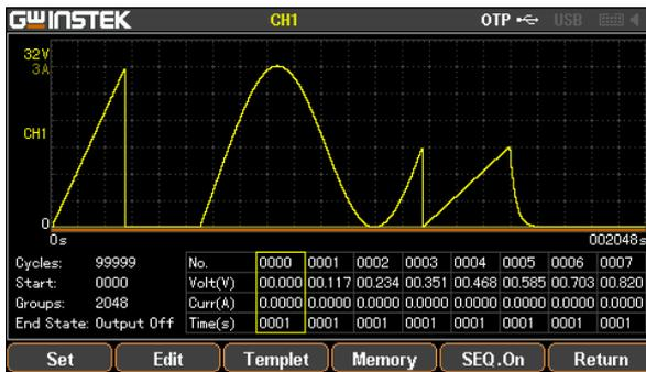
Output waveform of the GPP series
