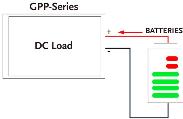
GPP-3610H and GPP-7250 are designed with a load function of up to 100W. GPP-3610H has built-in maximum 36.5V constant voltage load (CV), maximum 10.2A constant current load (CC) and maximum 1kΩ constant resistance load (CR) functions. GPP-7250 has built-in maximum 72.5V constant voltage load (CV), maximum 5.2A constant current load (CC) and maximum 1kΩ constant resistance load (CR) functions, so users can perform discharge tests without using an additional electronic load.
