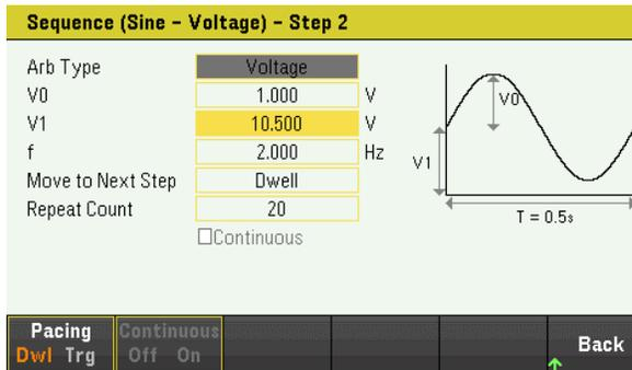
Figure 10. Change V1 from 7.5V to 10.5V for Step 2
