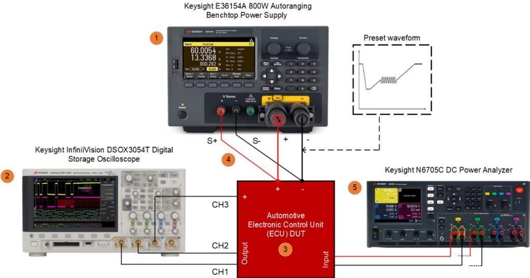
Figure 3. Simplified hardware connection diagram for the bench test.
