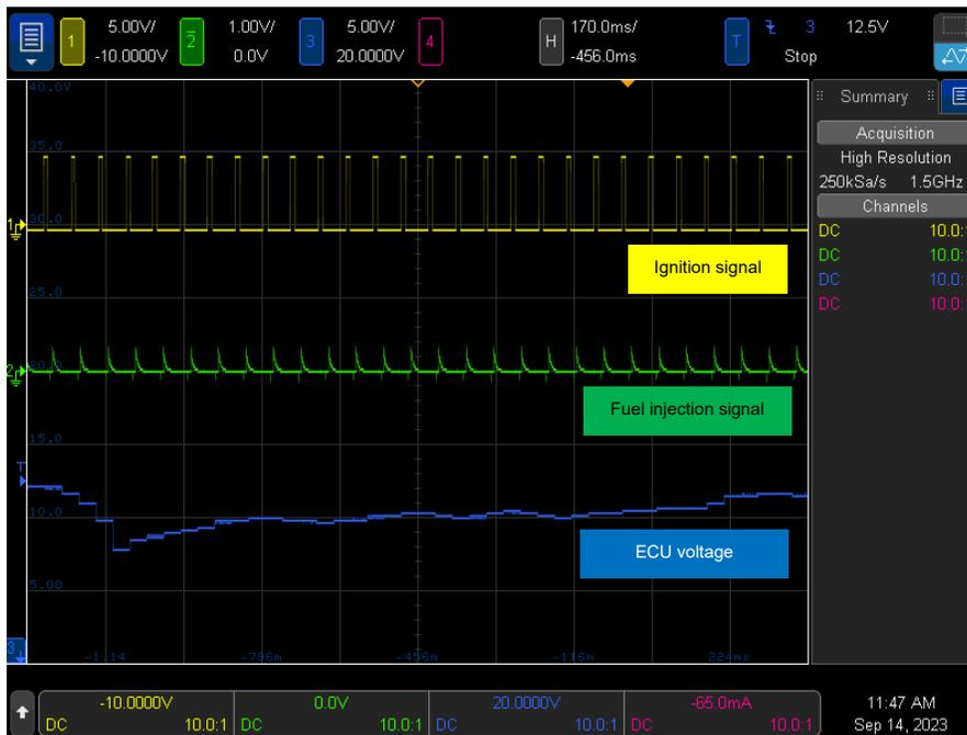
Figure 19. The input voltage, fuel injection, and ignition output signal of the ECU
