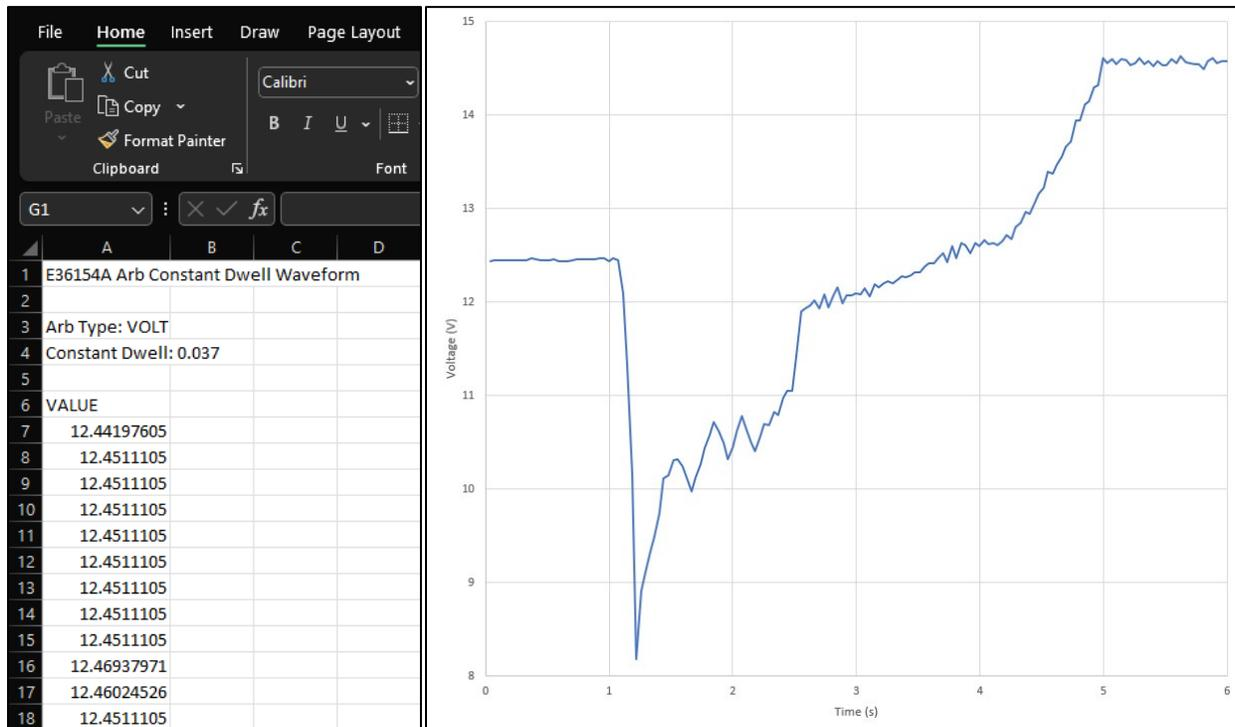
**Figure 15.** Vehicle voltage transient captured using an oscilloscope (right) and its CSV formatted data (left)
