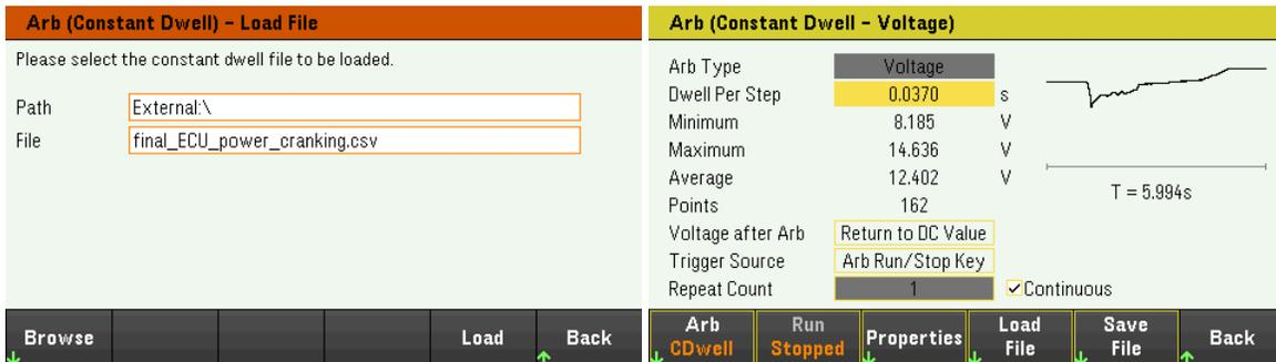
Figure 17. Power supply's file browser section (left) and summary of the imported waveform (right)
