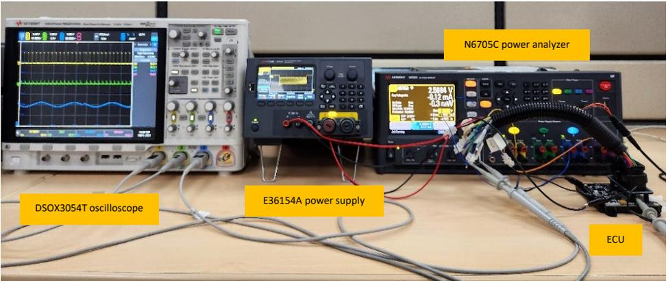
Figure 2. Hardware connection for the bench test.
