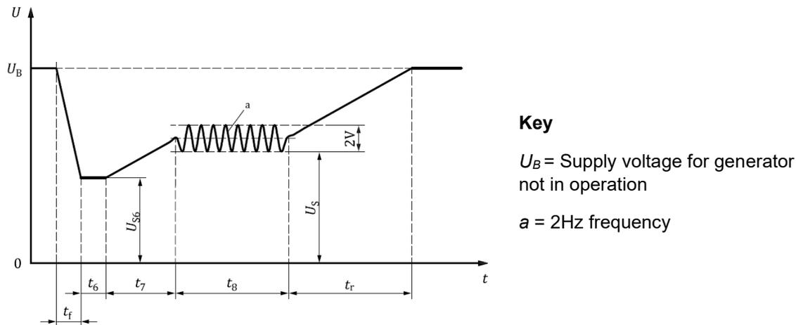
Figure 5. ISO16750 Starting Profile waveform.
