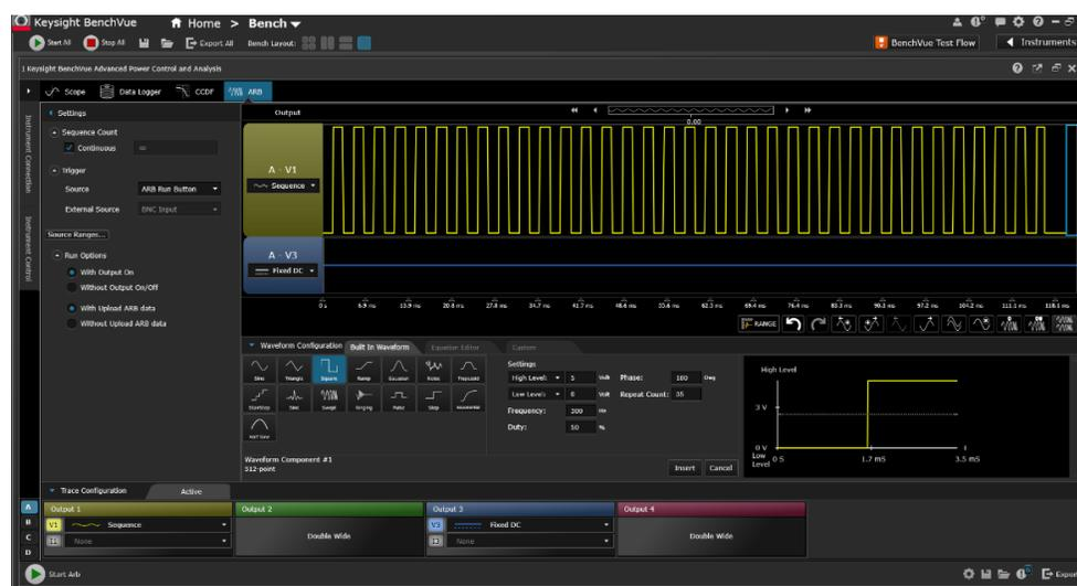
**Figure 4.** Emulating Cam tach and MAP/Oxygen sensor signals configured as V1 and V2, respectively, using the BV9201B software
