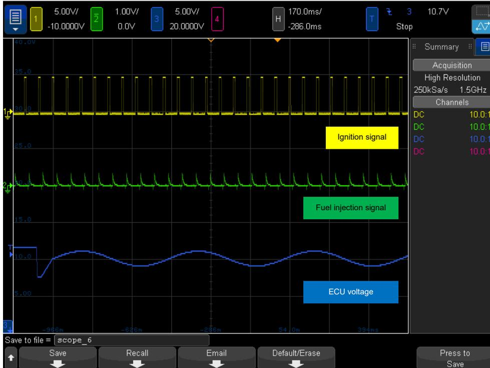
Figure 13. ECU input and output signals captured using the InfiniiVision oscilloscope
