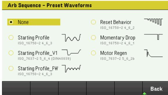
**Figure 6.** Available ISO waveform presets of the DC power supply.
