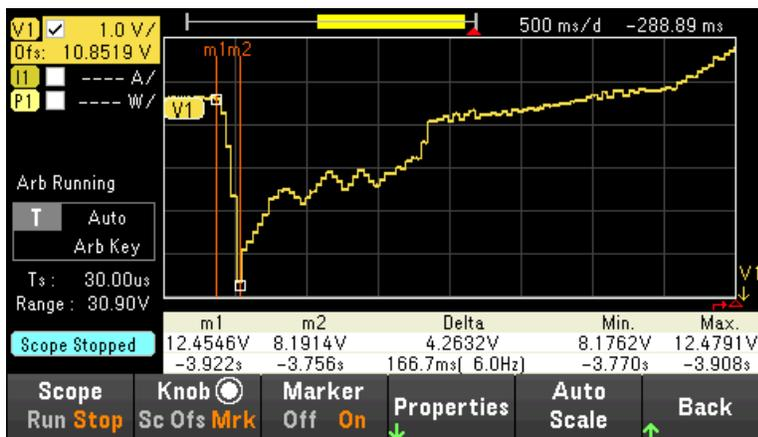
Figure 18. Voltage transient waveform captured using the E36154A power supply's Scope Mode
