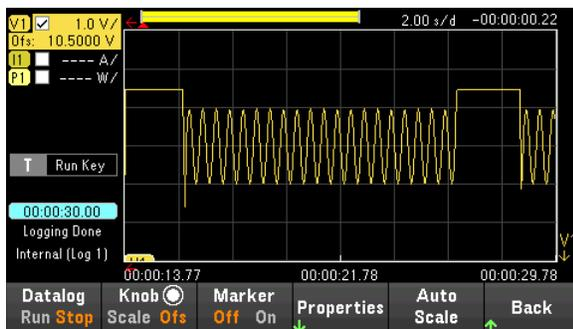
Figure 14. Starting Profile ISO waveforms captured using the E36154A Data Logger.
